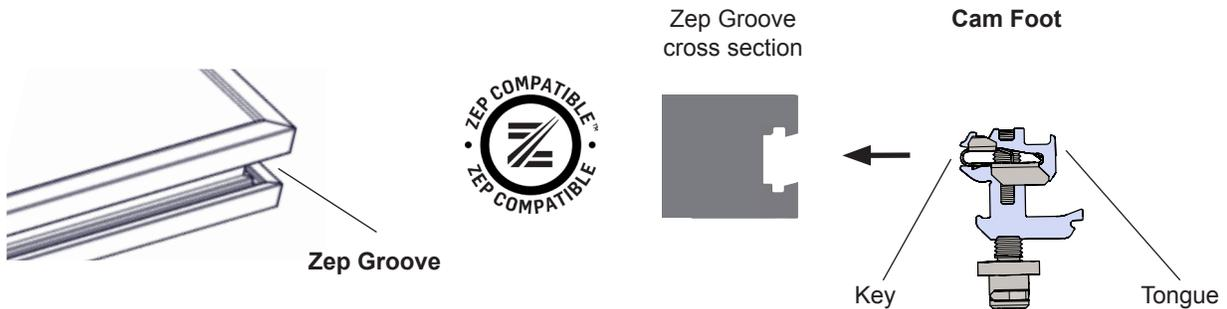
In ZS Ramp, the Key side of the Cam Foot inserts into the Zep Groove, securing the module in place. The locking process is auto-bonding.
